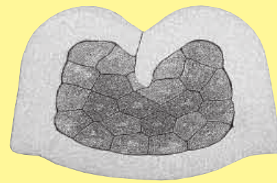
B shape cross section stamped contact
