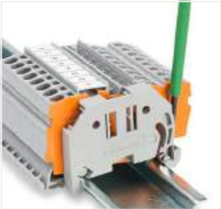
Removing an end stop from the DIN-rail.
