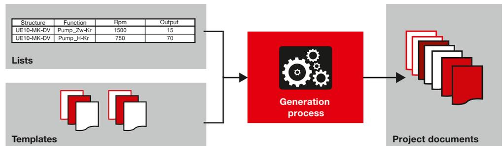
Fig. 14: Automated generation of design documentation based on templates
