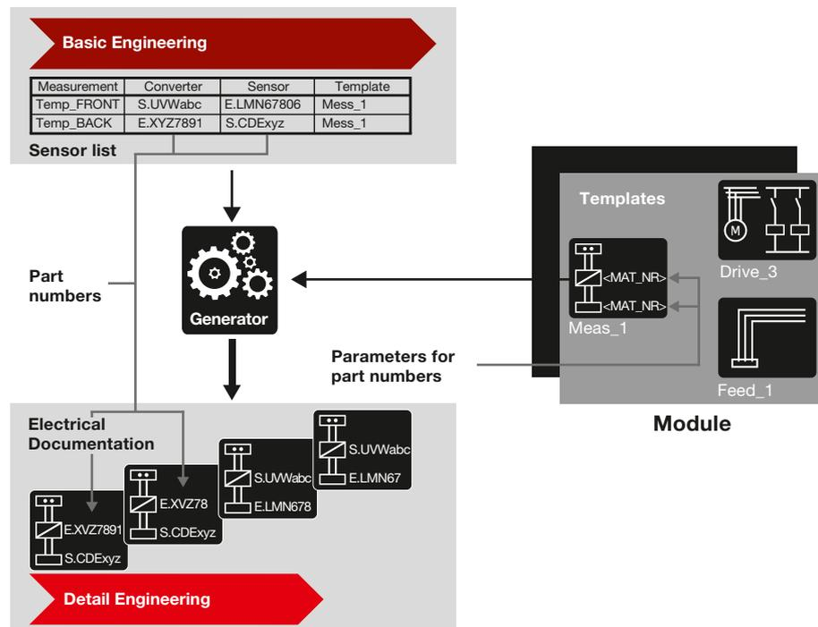
Fig. 21: Part number as a parameter: Decoupling parts and template
