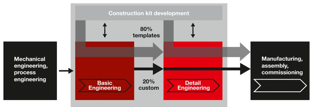
Fig. 2: Module-based engineering process in large plant design
