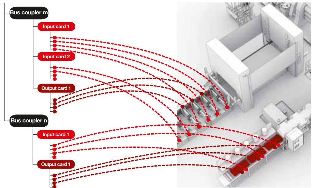
Fig. 7: Collection of signals and the design of control hardware
