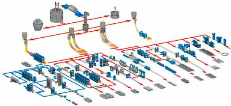
Fig. 3: Process chain for steel production (Source: SMS Siemag)
