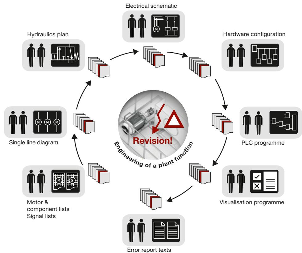
Fig. 13: Coordination and implementation workload for changes  $\Delta$
