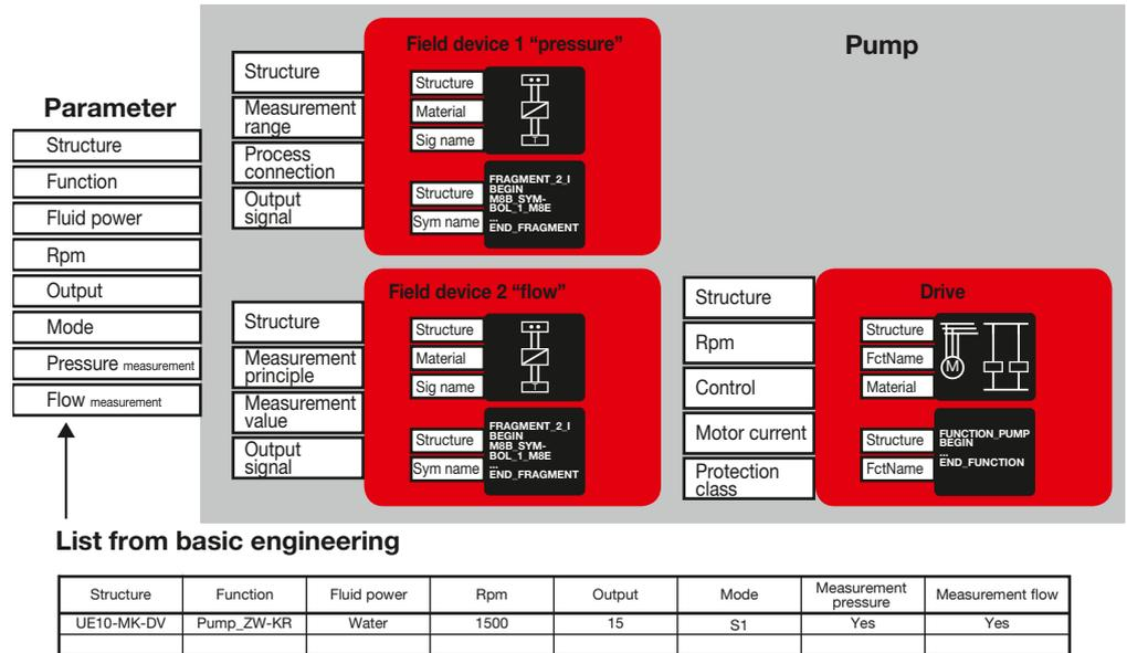
Fig. 20: Setting the parameters of functions and templates with data from basic engineering
