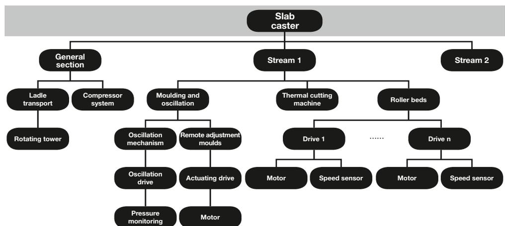
Fig. 17: Excerpt from the functional structure of a slab caster
