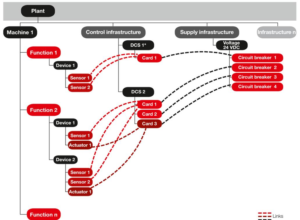
Fig. 8: Assigning signals to PLC cards and PLC cards to electrical supply (\*DCS – Distributed Control Systems)
