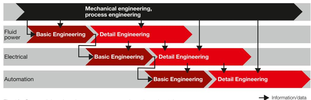
Fig. 10: Sequential engineering processes cause long throughput times
