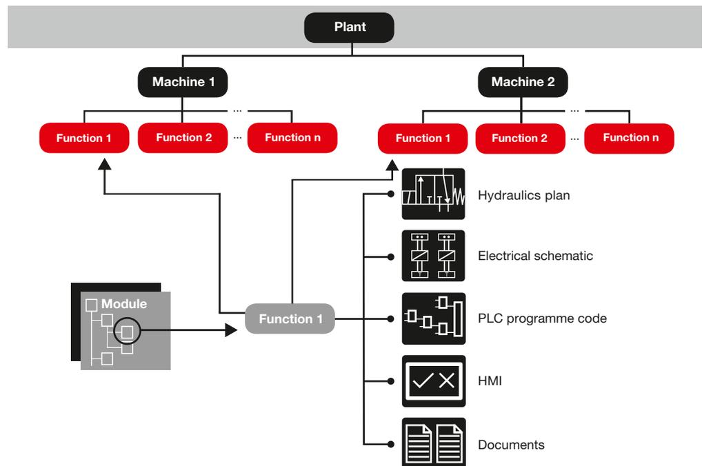
Fig. 18: Multiple use of interdisciplinary modular elements
